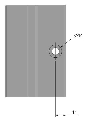
Hole in the wall adapted to the chosen screw
